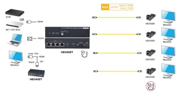
(2)Stack to another HE04SET through HDMI loop out port to get configuration of 1 in 8 out.
