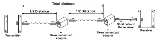
2. Recommend to change VE01R CAT5 receiver to VE02DALS, which built in RGB skew adjustment for the optimum video performance under long cable run. It also could be daisy chained for another VE02DALS to extended working range over 300 meters and multiple displays
