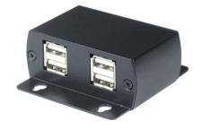
The UE04H USB extender design for extends 4 x USB device up to 50 meters from the location of your computer over CAT5/5e/6 UTP cable. It could eliminate the 5 meters distance limitation of USB. It is optimized for applications where two devices, such as the keyboard and mouse, must be operated remotely.
