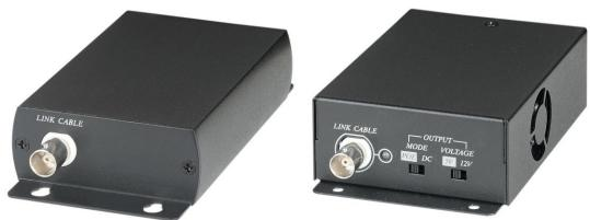
IP02P Extender is designed to send and extend IP or POE camera or any TCP/IP 10/100BaseT devices over existing coax cable. The distance could up to 180 meters by RG6U 75 $\Omega$  Coaxial Cable. They are completely transparent to protocols, codes, and applications ensuring compatibility with any IP, POE camera and its management software. It is perfect solution for sending IP Video links and Power to remote camera installation that are beyond the 100 meters distance limit of Ethernet.
