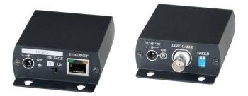
IP02EP IP extender is designed to extend any TCP/IP devices for long range transmission up to 500M over existing coaxial cable. The benefit could send power to camera use over same coax cable. It is perfect to add one IP camera with power over existing CCTV analog video camera environment. It is a great surveillance solution for sending IP video links to remote camera installation that are beyond the 100 meters distance limit of Ethernet and also provide camera power together.
