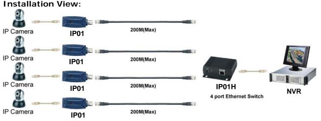
Caution: IP01H unit with BNC male terminator at channel 2, 3, 4. Do not remove the terminator if you do not use these channels. Otherwise, it will cause this Switch not working.
