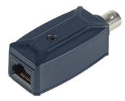
IP01 is a low cost and easy, speedy solution to allow you use existing coax cable to send IP camera signal. Used in pairs with your RG59 cable to exceed the IEEE 802.3 10BaseT specification. The working range could up to 200 meters at 10Mbps speed.
