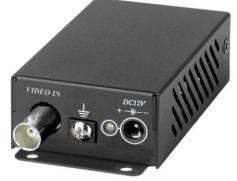
The GL001HD Video Ground Loop Isolator is an active devices which reduce ground loop interference without any video loss on HD CCTV signals. It could be easily install in a new or added to existing systems. It is useful where a video signal is transmitted via cable between points with different ground potentials, differences in ground potentials are typically caused by unbalanced power line loads.
