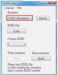
In main screen you will see the 「COM4 (Emulator)」 if the emulator have been connected with PC and installed driver properly
