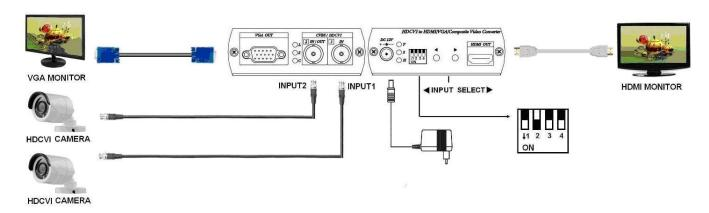
\* Allow two camera inputs with 2 outputs: HDMI, VGA as a switcher.
