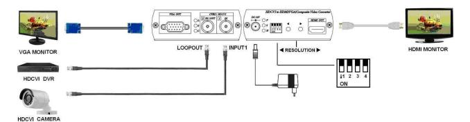
\* 3 outputs: HDMI, VGA, loop output as a distributor.
